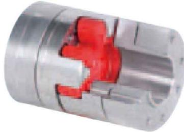
ROTEX® GS is a three-part, axial plug-in coupling backlash-free under prestress. It is convincing even with critical applications by its backlash-free power transmission, its stiffness which is each adapted to the application and its optimum damping of vibrations. This principle of installation offers significant assembly possibilities which optimize the assembly times in production.
