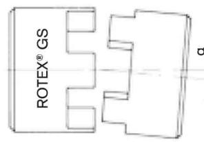
Due to its design the ROTEX® GS is able to absorb axial, angular and radial displacement, without causing any wear or premature failure of the coupling. As the spider is only stressed under pressure it is ensured that the coupling will remain backlash-free even after a longer operation period.
